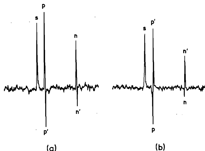
FIG. 2. The 15 N nmr spectra ( t = 6.5 min) during the simultaneous rearrangement of 2,6-dichloro- N -nitroaniline and 2,6-dibromo- N -nitroaniline under the conditions defined in Table 3: (a) with the label in the dichloro compound; (b) with the label in the dibromo compound. The lettering follows that in Fig. 1 with the dashed symbols (n', p') indicating the nitramine and product from the dibromo series.
