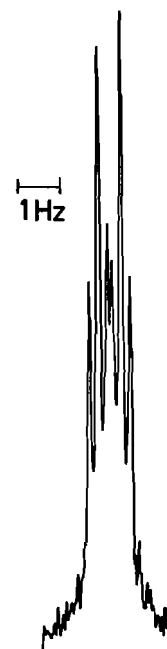
FIG. 4. One multiplet of the INEPT spectrum of the methyl {}^{13}\text{C} nucleus of a 2 mol% solution of 2,6-dibromoanisole in acetone- d_6 at 300 K and 75.486 MHz. The large splitting arises from coupling to the para proton and is 0.541(5) Hz in magnitude. The triplets arise from a coupling of 0.217(5) Hz to the meta protons.
